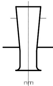
Such a front-end is chosen for the HSM 814, with for 4 orifices. By performing the calculations it can be shown that each of these orifices could be approximately 62.5 mm in diameter. The distance to the throat of the chimney could be 370 mm, the straight mixing section 355 mm and the conical diffuser above 1046.5 mm. The total provides an overall
