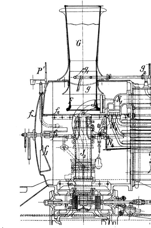
In the adjacent figure, the diffuser chimney is drawn in. It fits (of course) in the original outside chimney which should be extended slightly.
